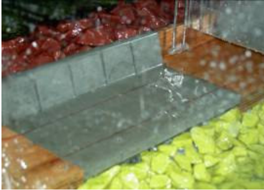
Figure 8. Crown-wall during 2D physical model testing (view from rear side).
