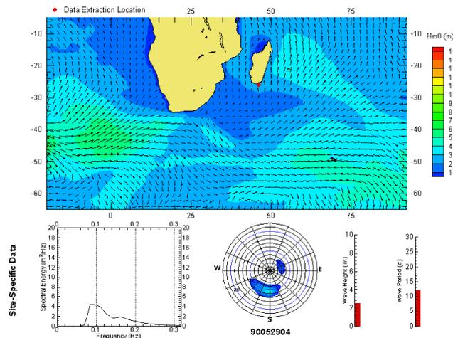
**Figure 4 – Sample Output from WaveWatchIII Model**
