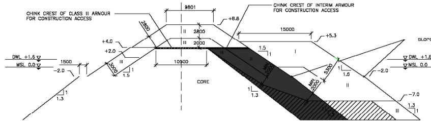
**Figure 7 – Preliminary Design Cross-Section for Breakwater**
