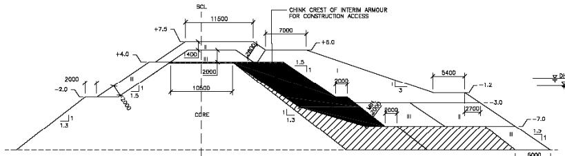
**Figure 11 – Final Design Cross-Section for Breakwater**
