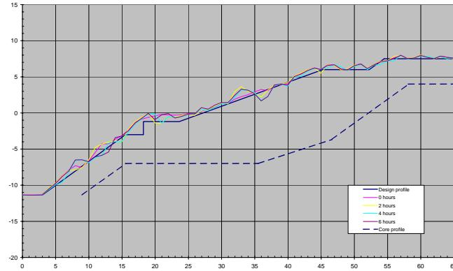
**Figure 10 – Profile Measurements During Final Test of Full Cross-Section**
