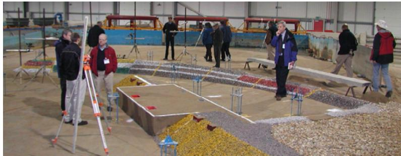
**Figure 8 – Overview of 1:50 Scale Model of Breakwater and Port**
