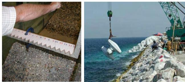
**Figure 6 – Simulated Crane Placement in Model and Actual Placement**
