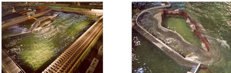
Figure 33. 3D physical model test for the Perimeter Breakwater Escombreras. CEDEX.
