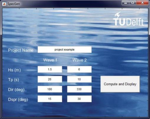
Figure 1 SpecGen Start-up and Computation Window
