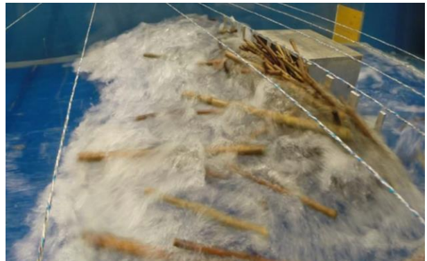
Figure 4. Combined debris and hydrodynamic loading due to dam-break/bore impact: (a) Nistor et al. (2021); (b) Wüthrich et al. (2020b), considering only (natural) driftwood.
