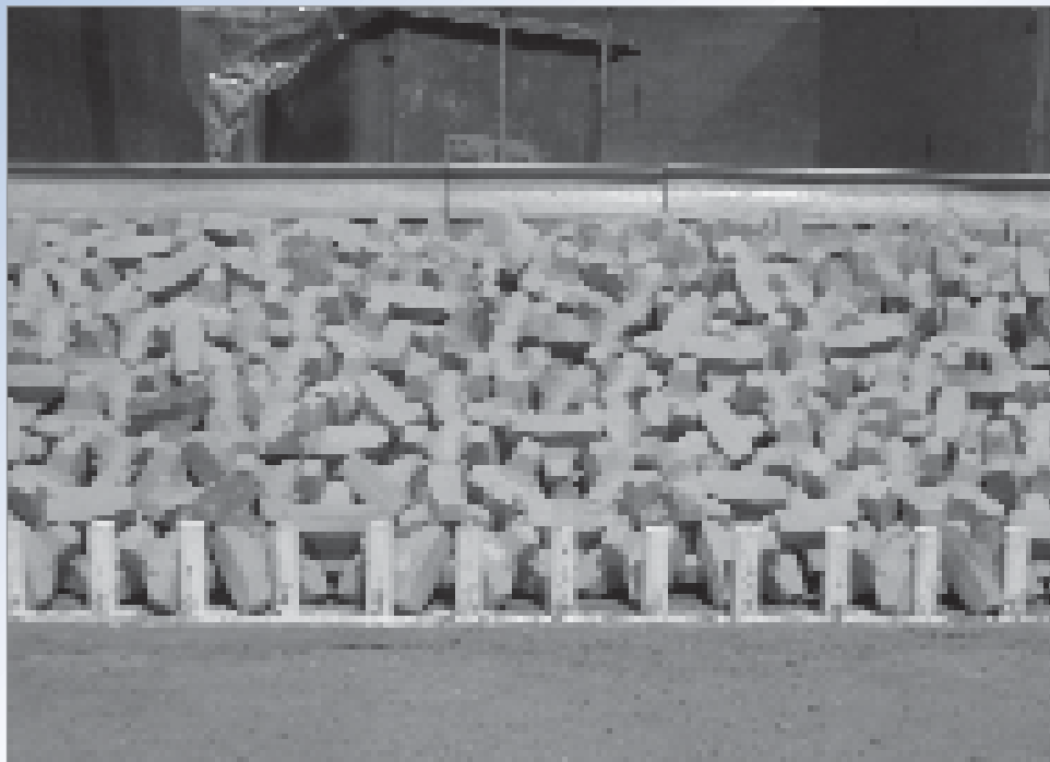
Figure 6.20 View of the model test for typical toe detail using concrete piles (courtesy HR Wallingford)
