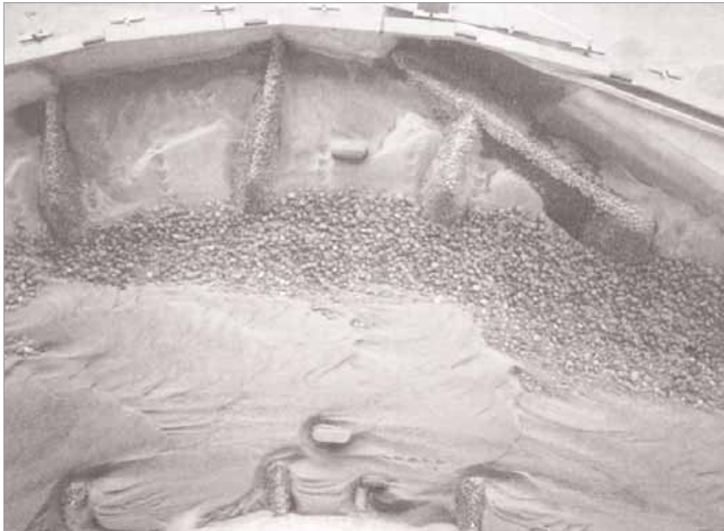
Figure 4.91 Example of a physical model of a river with mobile bed
