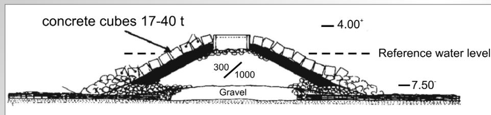
**Figure 10.21** Modification after construction: adding concrete cubes
