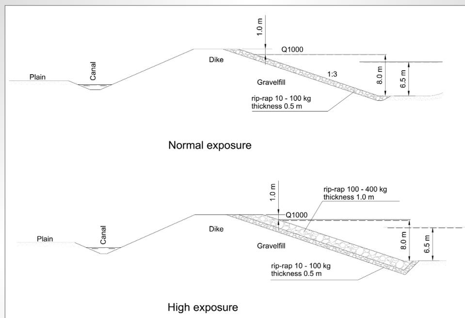
**Figure 10.20** Modifications to bank protection on the River Rhône
