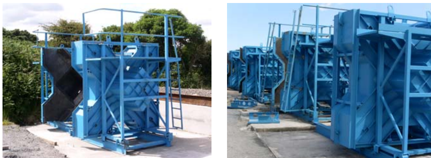
Figure 5: Xbloc moulds, 4 m 3 size.
