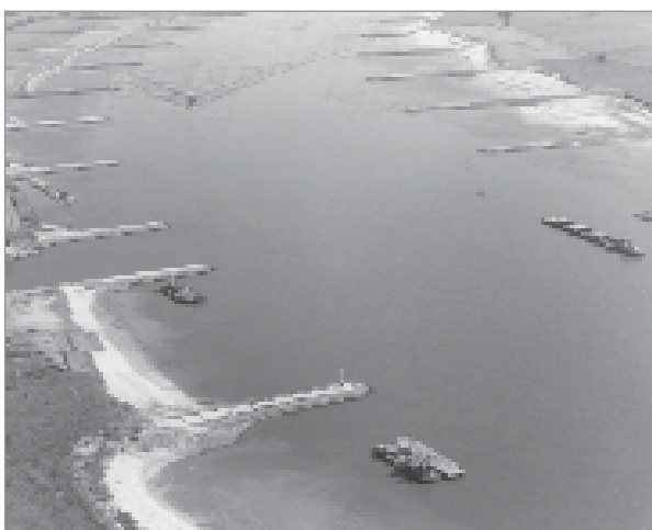
Figure 1.17 Spur-dikes (after CUR 1995)
