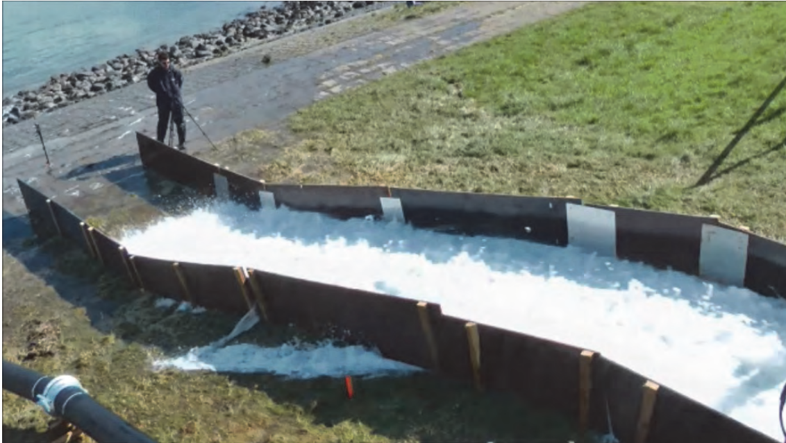
Figure 3.8 Snapshot of a three-minute video showing the overtopping wave volume from the wave overtopping simulator from above
