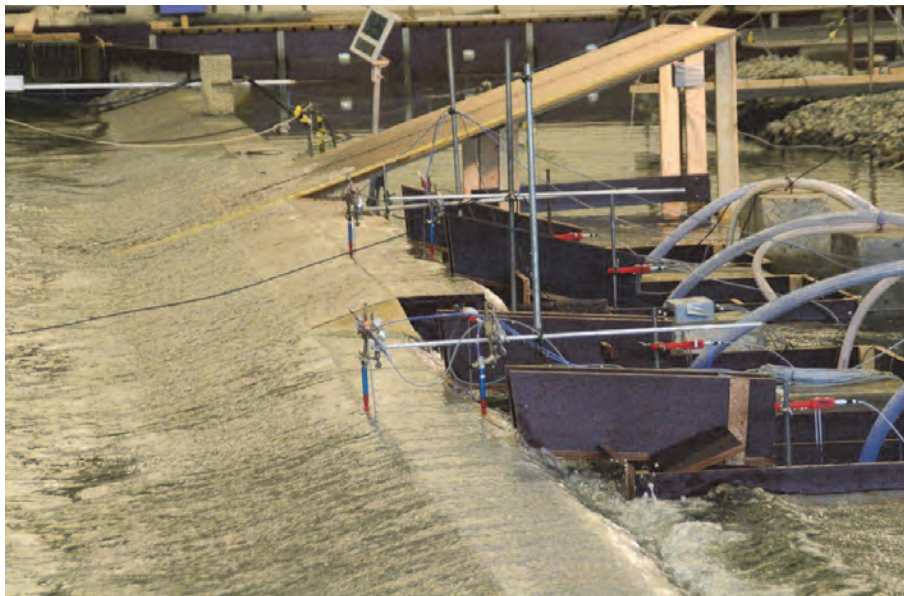
Figure 4.31: Measuring wave overtopping at four locations (four chutes leading to an overtopping box) and at two crest levels; measuring flow velocities on the crest with micro-propellers (blue with red) and flow depth with small wave gauges (next to the micro-propellers). Wave run-up was measured by a capacitance wire along a non-overtopped slope (upper middle). Set-up at wave basin at DHI, DK
