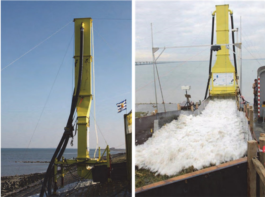
Figure 4.40 The Wave Run-up Simulator
