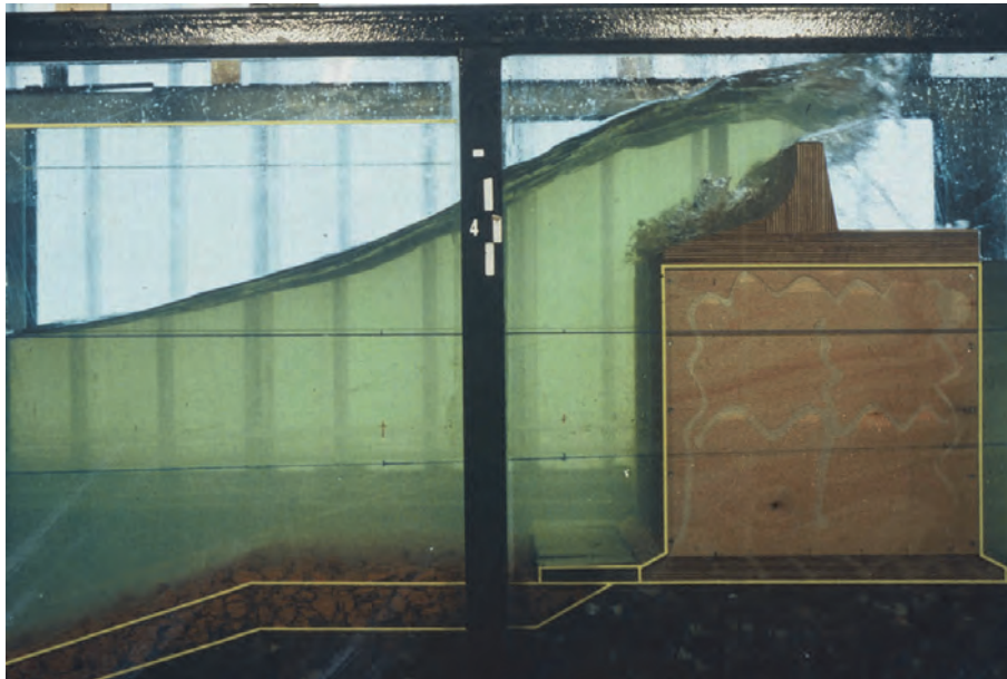
Figure 4.27: Massive wave overtopping simulated in a wave flume on scale 1:50. Wave flume at Deltares, NL
