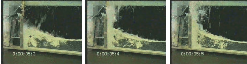
Figure 7.4: A broken wave at a vertical wall, resulting in a broken wave overtopping condition
