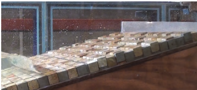
Figure 5.33: Testing block pattern on a scale of 1:22. Courtesy Deltares
