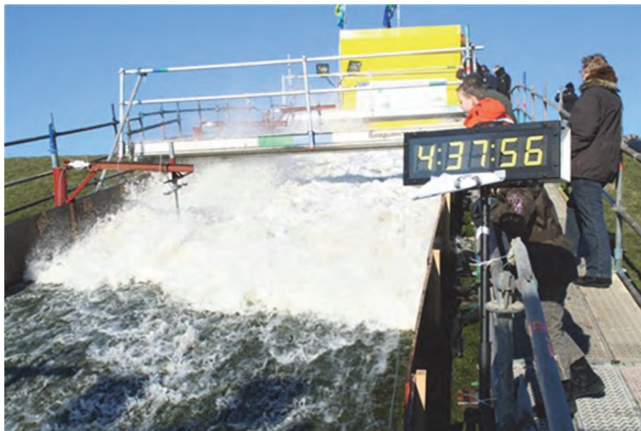
Figure 4.34 Release of a large overtopping wave volume
