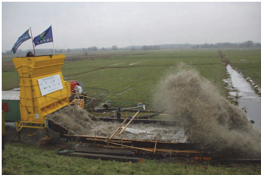
Figure 4.36 Measuring wave forces on vertical plates under flows from the Overtopping Simulator
