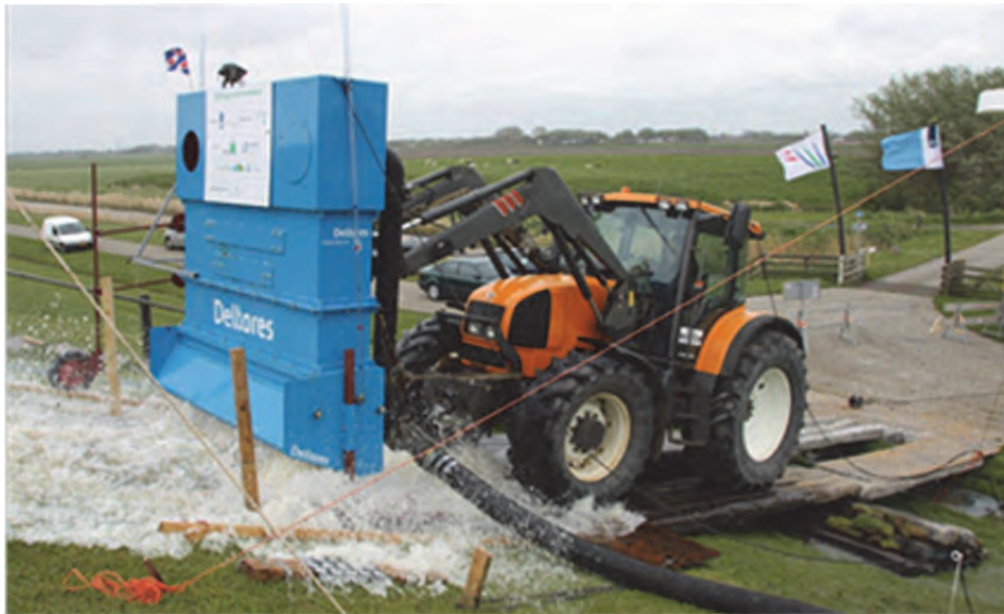
Figure 4.42 Test with Wave Impact Generator
